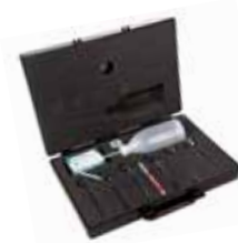
6 Poreusheid test, Karsten Pipe test kit
